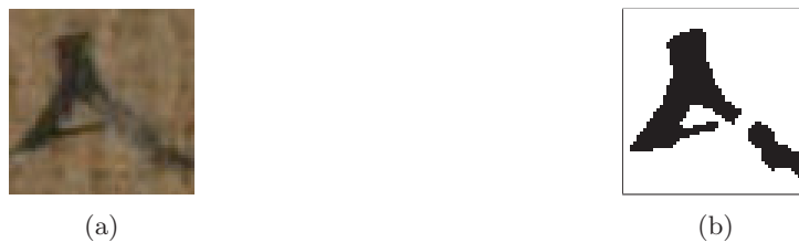
Figure 3.3: Original alpha \alpha in 3.3a and alpha \alpha after Otsu's binarization in 3.3b
