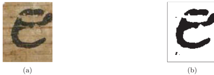
Figure 3.4: Original epsilon \epsilon in 3.4a and epsilon \epsilon after Otsu's binarization in 3.4b
