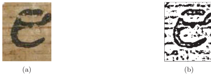
Figure 3.2: Original epsilon \epsilon in 3.2a and epsilon \epsilon after adaptive thresholding in 3.2b
